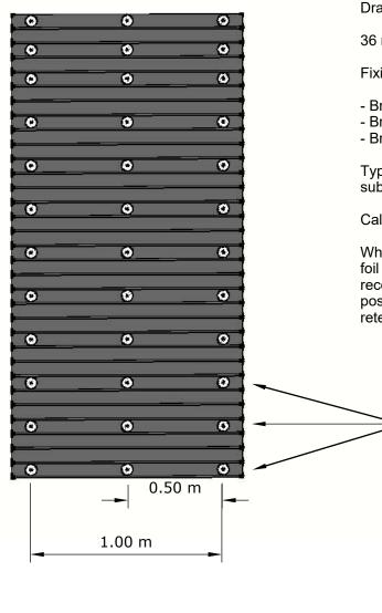
Drawing shows recommended fixing points for brick slip tracking system.
